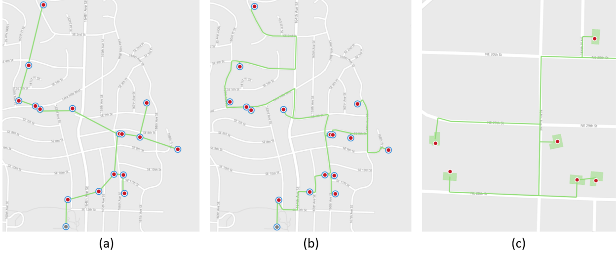
Figure 3: Sample output from the system (a) MST of required entities, (b) Fiber network layout using existing road network (c) Close-up of an output fiber network
